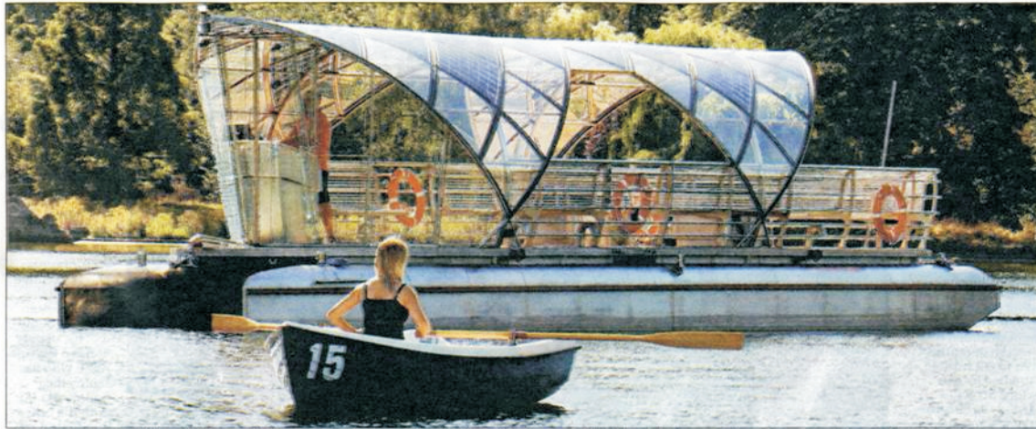
Silent mover: the Solar Shuttle on the Serpentine has a roof made from 27 glass panels that collect energy from the sun and use it to power the boat
